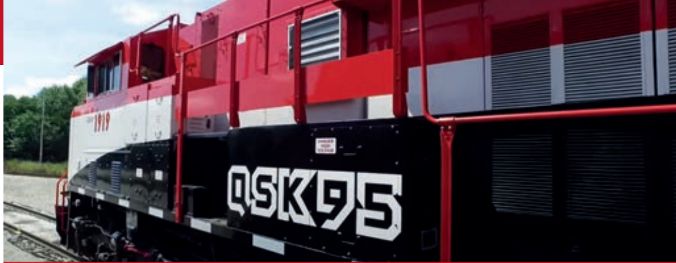
Rail has been an key segment for Cummins Tier 4 high horsepower diesels. A QSK95 diesel has been in test with the Indiana Rail Road and Amtrak is using the engine in new Siemens Charger locomotives.
